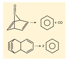
Two chemical reactions, both fragmentations yielding benzene (the first from norbornadienone, the second from a benzene dimer) are highly exothermic, giving off an energy of about 215 kilojoules per mole. Yet they both have substantial barriers (about 65 kilojoules per mole) to proceeding, sufficiently high that it is possible to isolate the two.
